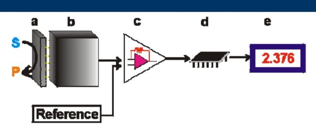
Schematic diagram showing the main components of a biosensor. The bio-reaction (a) converts the substrate to product. This reaction is determined by the *transducer* (b) which converts it to an electrical signal. The output from the transducer is amplified (c), processed (d) and displayed (e).
